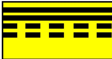
**3.3.4. Markings.** Pavement markings on taxiways are always **yellow**. The taxiway centerline is painted on all taxiways. On the edges of some taxiways, there is a solid, double yellow line or double-dashed line. If pavements are usable on both sides of the line, the lines will be dashed; if not, the lines will be solid.
